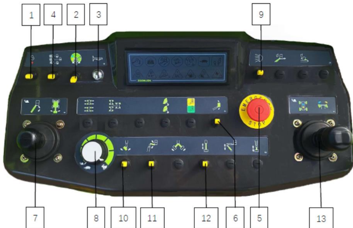
Figure 2-12 Platform Control Panel (Only the switch number corresponding to the existing function is identified).
